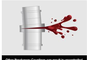
Other Breakaway Couplings can result in uncontrolled spillage in the event of a partial separation.
